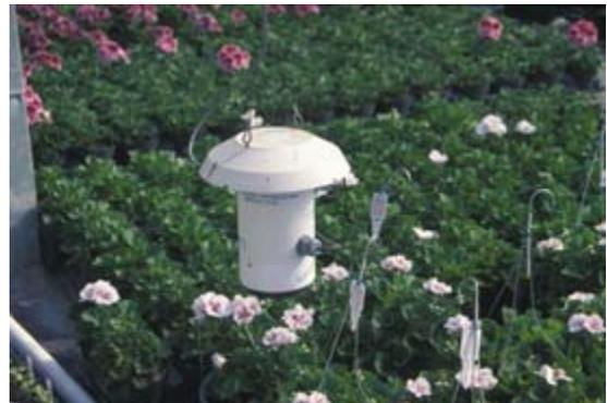
**Thermostats** are of two types: on-off and proportioning. Both are inexpensive and easy to install. On-off thermostats control fans, heaters and vents with a change in temperature. Proportioning devices provide continuous control of systems with temperature changes.
